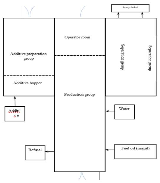
The dimensions of the "Fluff Preparation Block" and the "Separation Block" are 6000x2450x2450mm
